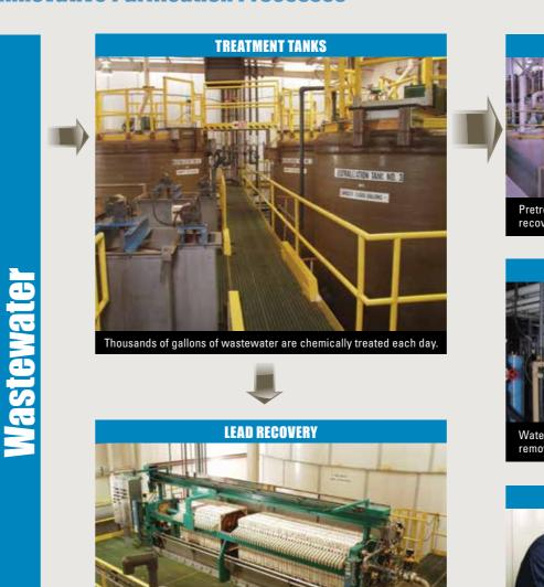
olids are removed, smelted and refined for lead recovery.
