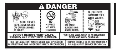
It never needs watering, and should never be opened as this would infuse the battery with excess oxygen from the air. In addition to damaging the battery, opening it also voids the warranty.
