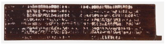
Competitor's plate formed in the battery case. White areas indicate plate is not fully formed.
